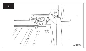
3.3 Remove the two fixing screws from the pilot bracket, see diagram 3. Gently draw the assemble away from the firebox to give access to the nuts and ignition lead.
